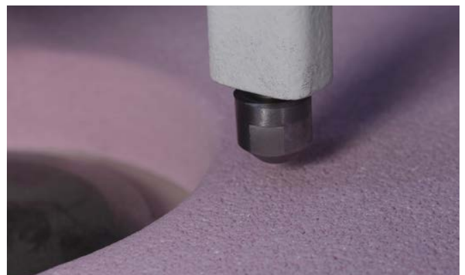
Automatic dressing of the grinding stone
